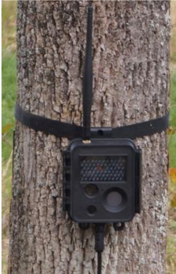
Fig. 5. BuckEye X7D camera trap with wireless functionality, here shown without protective housing.
